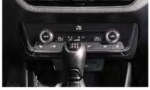
DUAL ZONE AIR CONDITIONING WITH CLIMATRONIC ELECTRONIC CONTROL
