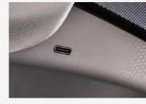
ROOF PANEL USB Located in the roof panel at the rear-view mirror, this optional USB-C port is ideal for charging devices mounted on the windscreen.
