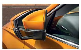
ELECTRICALLY ADJUSTABLE, HEATED AND FOLDABLE AUTO-DIMMING DOOR MIRRORS
