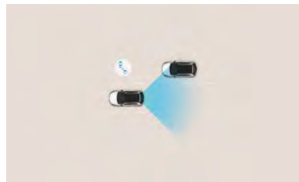
Blind-Spot Collision Warning (BCW): Radars detect traffic in the vehicle blind spot, warning drivers with an audible alarm when the indicator is used so you can be aware of the traffic around you even when you can't see it.
